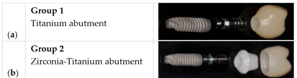
Figure 4. View of the constructive sample of the two groups: (a) group 1 and (b) group 2.
