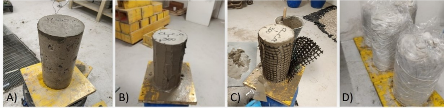
Fig. 1. Steps of the FRCM confinement jacket application on the cylindrical concrete specimens.
