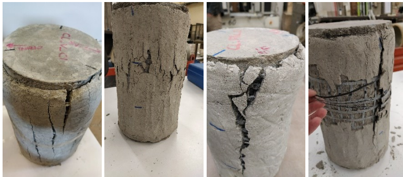
Fig. 3. Crack pattern observed after testing.
