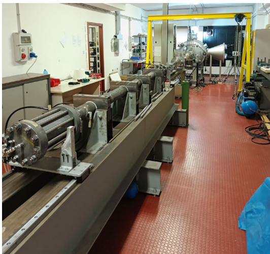
Fig. 1 Two stage light-gas gun in the hypervelocity facility of the University of Padova
