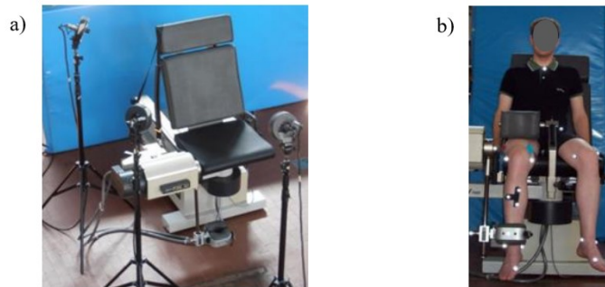
Fig.1. a) Technogym REV 7000 and BTS optoelectronic system (only three cameras are shown); b) Markerset, electrodes and testing conditions.
