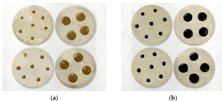
Figure 1. Samples for DSR testing: SB (a) and BB (b).
