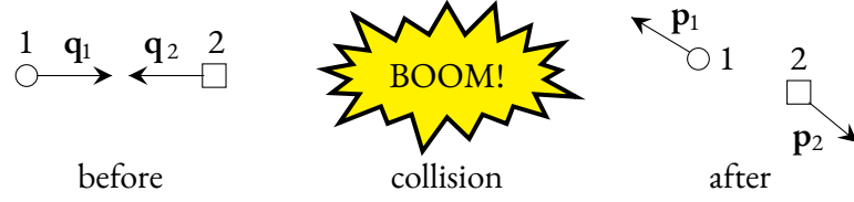
Figure 1.4: A collision of a particle 1 with initial three-momentum \mathbf{q}_1 and energy \mathcal{E}_1(q_1) with a particle 2 with initial three-momentum \mathbf{q}_2 and energy \mathcal{E}_2(q_2) . Here, the effect of the collision is just that of modifying the three-momentum of the particles (i.e. it is not an annihilation or a creation process), so that, after the collision, the particles have three-momenta \mathbf{p}_1 and \mathbf{p}_2 , and their energies are \mathcal{E}_1(p_1) and \mathcal{E}_2(p_2) , respectively.
