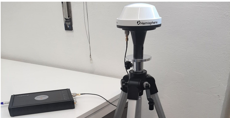
FIGURE 4.4: Setup used for the experimental dataset collection: Septentrio PolarRx5 receiver connected to an A42 Hemisphere antenna.
