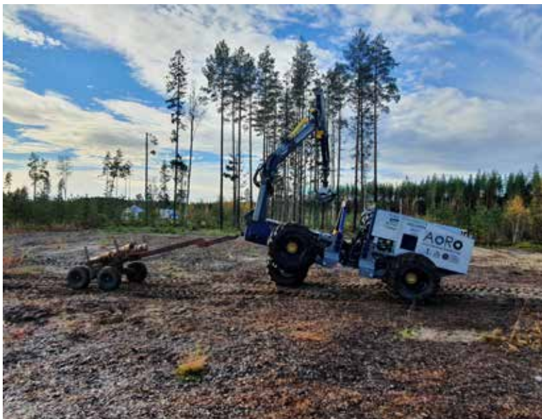
Figura 8.36. Prototipo di forwarder autonomo sviluppato dall' Arctic Off-Road Robotics Lab (AORO) in collaborazione con Luleå University of Technology, Swedish University of Agricultural Sciences e The Cluster of Forest Technology (fonte: AORO)
