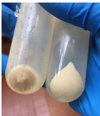
Figure 21. Washing process of the inclusion bodies. The crude insoluble fraction of the bacterial lysate (left tube) is washed multiple times in presence of detergent to isolate the inclusion bodies (tube on the right).
