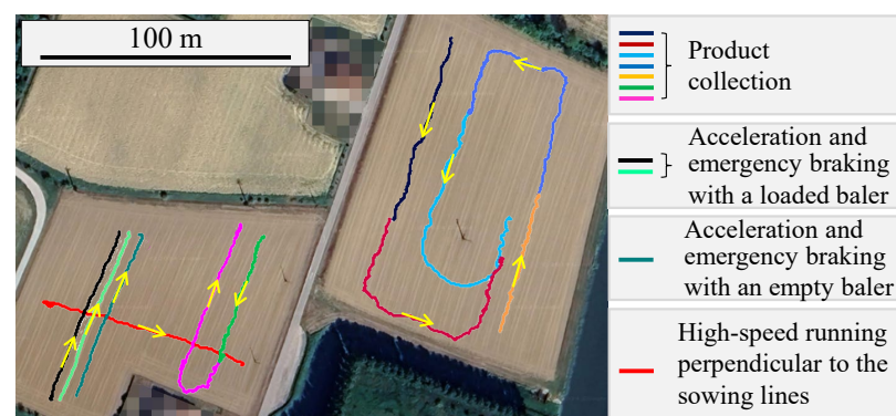
Figure 10. Satellite image of the fields where the load acquisitions took place; the routes followed by the baler during the different acquisitions are reported.
