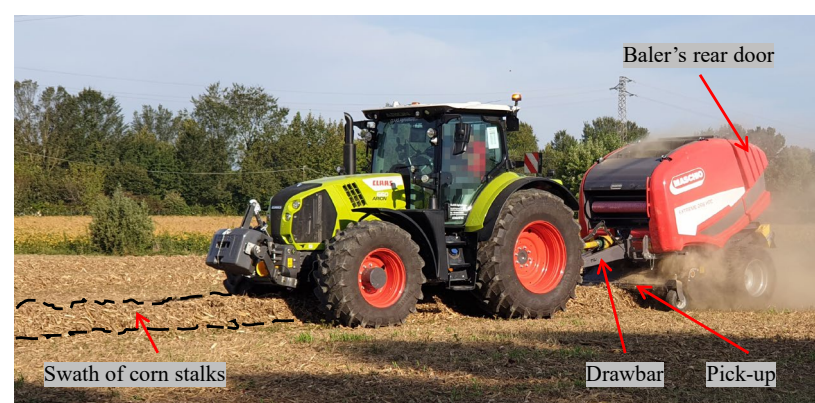
Figure 11. Round baler with the product collection mechanism (pick-up) deployed during the in-field load acquisitions and towed by a Claas Arion 660 tractor.
