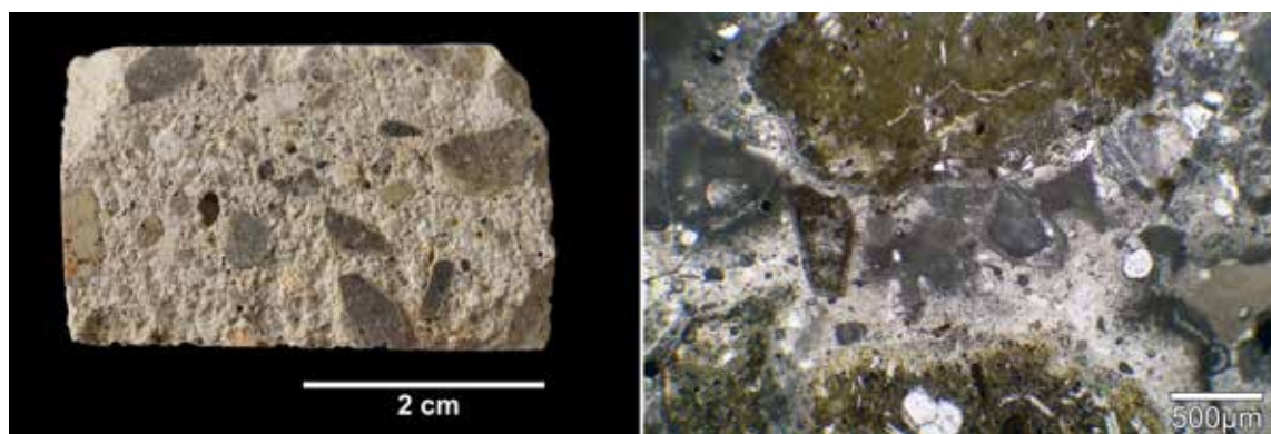
Fig. 9. (left) Cross-section of a mortar sample enriched with volcanic pozzolan from the Euganean hills from the masonry structures of the theatre of Montegrotto; (right) micrograph of transmitted light (parallel nicols) of reacted volcanic aggregates (breccias) (photos by Simone Dilaria).
