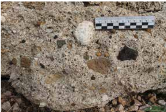
Fig. 7 - Volcanic pozzolans (mainly pumices and fragmented tuffs), probably from the Gulf of Naples, in the bedding of the parietal opus sectile of the Temple of Aesculapius in Nora (3 rd century AD) (Dilaria in press).
