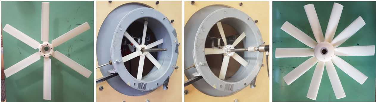
Figure 3: 3D printed rotor of the 14REF model fan (left), 20REF and 20R0B5 models mounted on the test rig (middle left and middle right), 20R0B10 model fan rotor (right).
