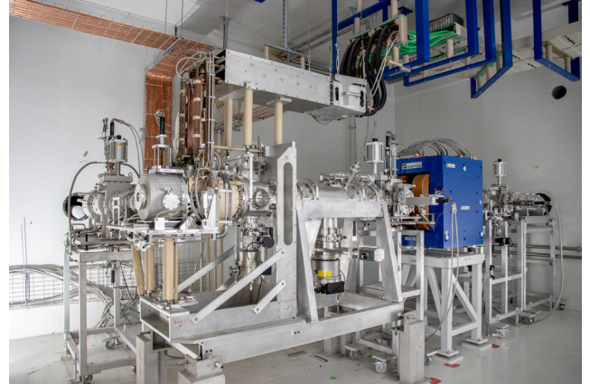
Fig. 2. View of the SPES Front-End and the RIB line within the ISOL bunker (S018).
