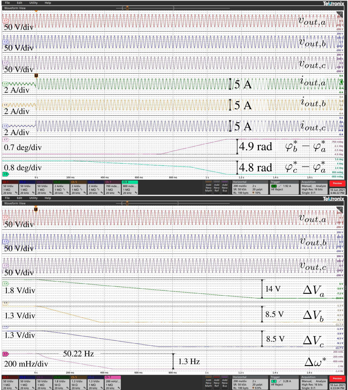
Fig. 4.12 Experimental results with EPC 1 in Fig. 4.6 implementing the proposed control scheme in Fig. 4.4. Transition into the islanded operation of EPC 1 and EPC 2 with balanced load of 12.5 Ω and grid frequency of 50.22 Hz.
