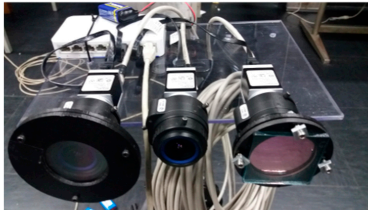
Figure 4. The multi luminance meter (on the right) and the multi-spectrometer (on the left); the color RGB camera is in the center.
