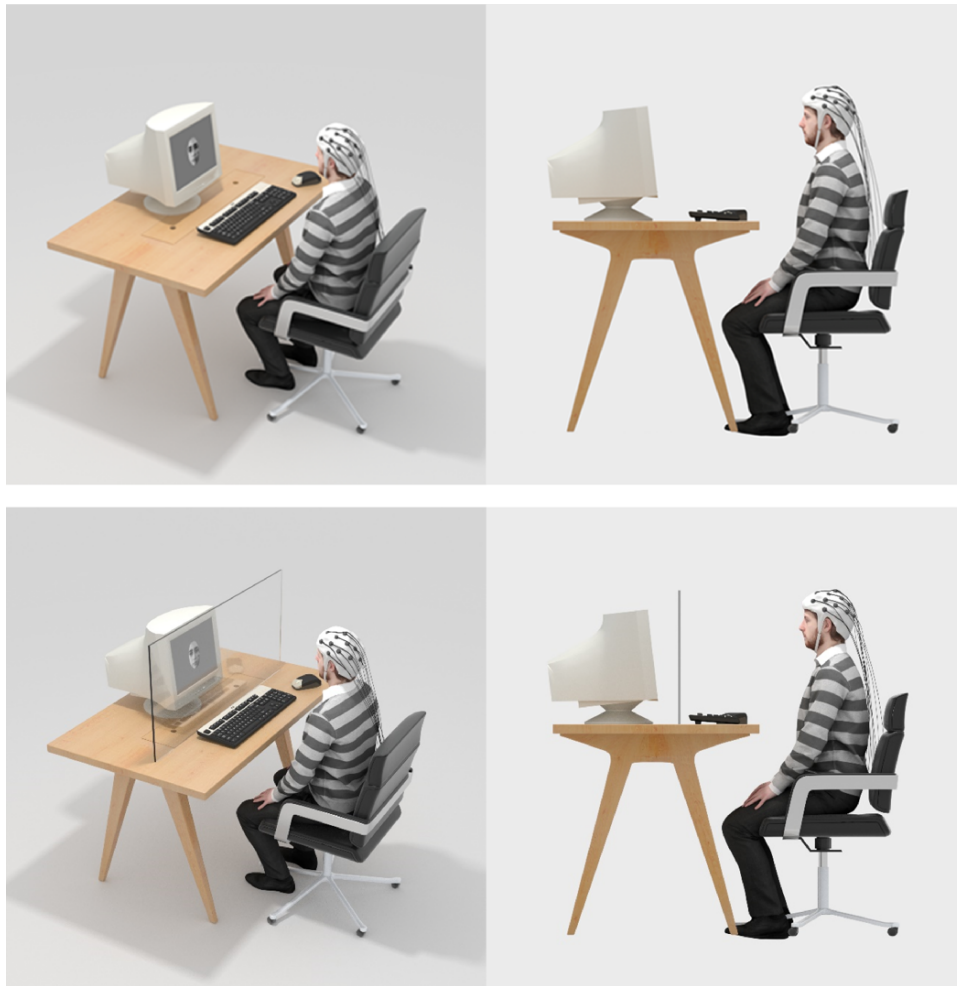
Fig. 1. Experimental setup, including the no-barrier condition (top) and the barrier condition (bottom).
