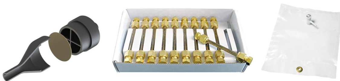
Fig. 5 Elements of the sampling system; starting from the left PM filter, desorption tubes (Photo by RESTEK) and sampling bag (Photo by RESTEK)
