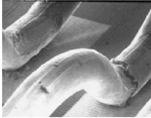
Fig. 17: Heel cracking in a double wire bond [36].
