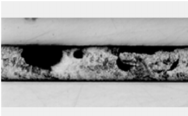
Fig. 22: Voids in the solder between ceramic substrate and base plate (SEM image, 100x) [42].
