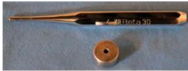
Figure 1. Stainless steel mold containing an opening hole with a diameter of 4 mm and a length of 10 mm, and a Beta tool for removing samples from the cylinder.
