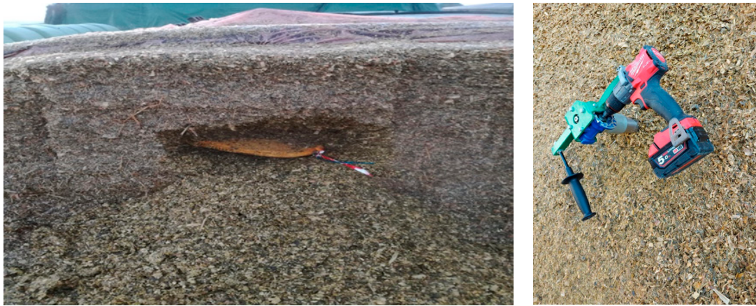
Figure 1. A net-bag buried in a bunker silo (left); the electrical probe (right) to collect a determined volume of whole-plant maize (WPM) silage used to calculate dry matter density and porosity.
