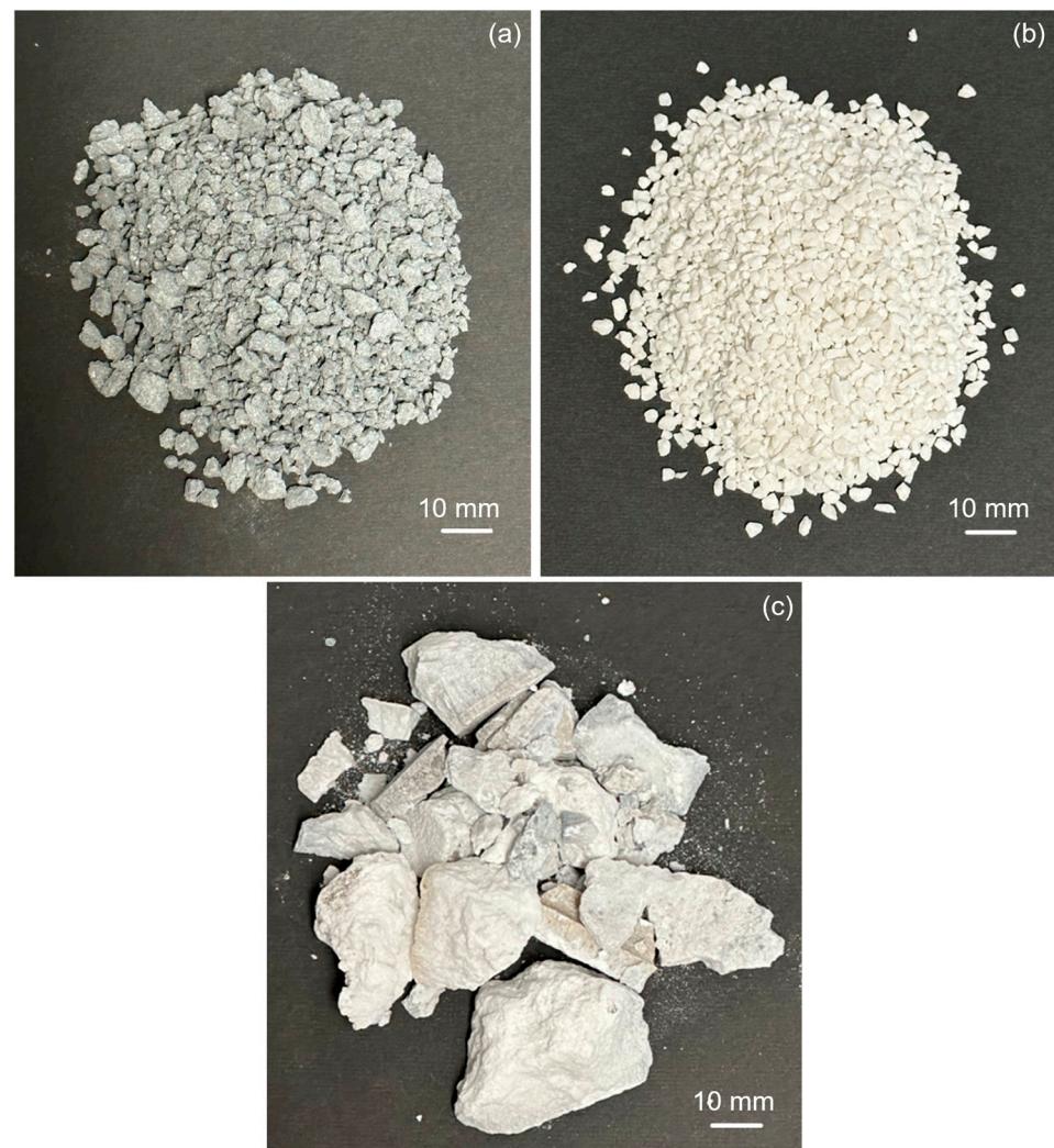
Figure 8. Granulated salt fluxes: (a) medium-sized drossing granulated flux, (b) fine-sized drossing granulated flux, and (c) coarse-sized granulated flux for scrap remelting.
