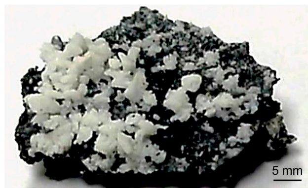
Figure 7. Non-reacted solid drossing flux granules on a dross lump.
