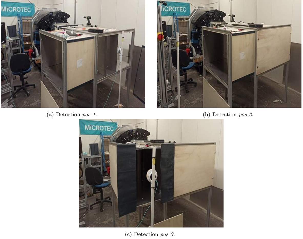
Figure 4.13: Photographs of the external shielding apparatus for Mito500 built in the bunker corresponding to the three positions presented in Figure 4.9. The measures are taken with the RaySafe 452 dosimeter.
