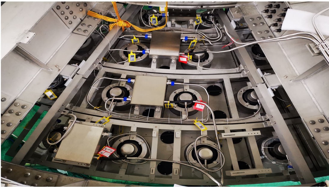
Figure 5.13. Picture of a sector of the stainless steel structure with three Underwater Boxes installed on the detector. Each box is connected to three 20-inch PMTs, whose bases are also visible.
