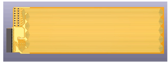
Fig. 11. Simplified detector design used for the Development Model of the sensor. The diodes are placed in the top-left edge of the board and the stack connector to the control electronics in the bottom-left edge. The 64 sensitive lines are arranged using an “S” pattern to cover the entire sensitive area.
