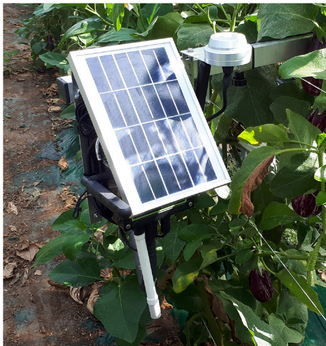
Fig 2. The Evja station. The Evja station hosting persistent sensors.
