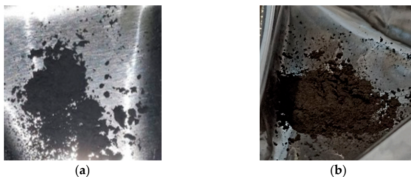
Figure 7. Pictures of the enriched 49 Ti (a) and 50 Ti (b) powders after the cryomilling process.
