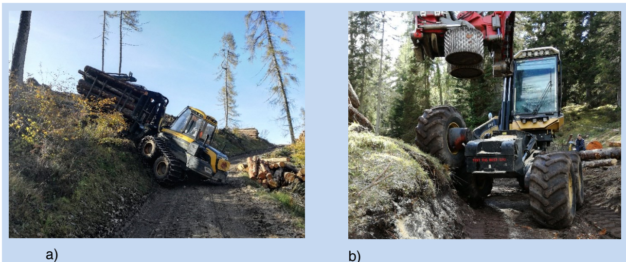
Figure 1.2 - Example of winch-assist forwarder working in steep terrain (a) and harvester with balanced bogie and hydraulic pendulum arms and axles equipped with a hydraulic cylinders (b)
