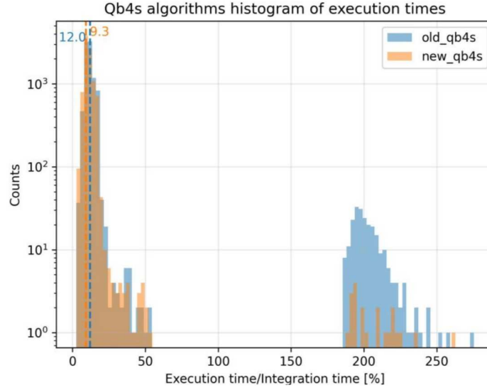
FIGURE 3.5: Comparison between the old and new algorithm in terms of computation time performance, calculated on a fixed experimental set of data.
