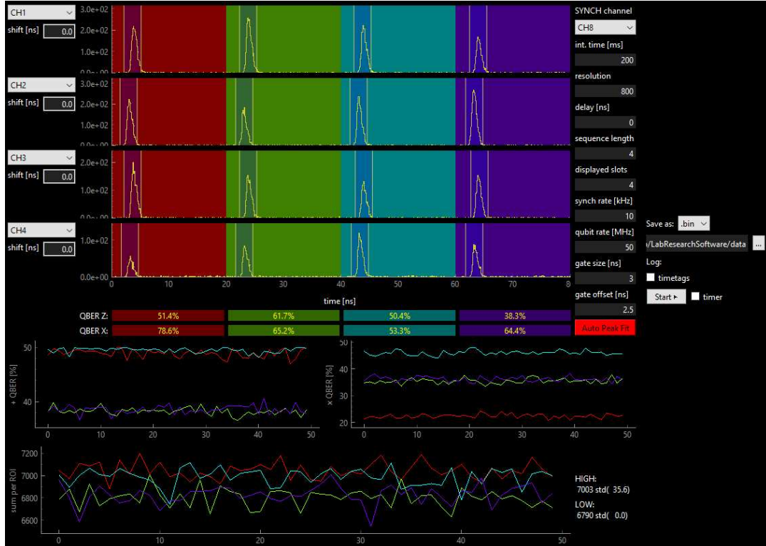
FIGURE 3.3: Detail of the software showing the QBER and total detections. Logging widget on the right.
