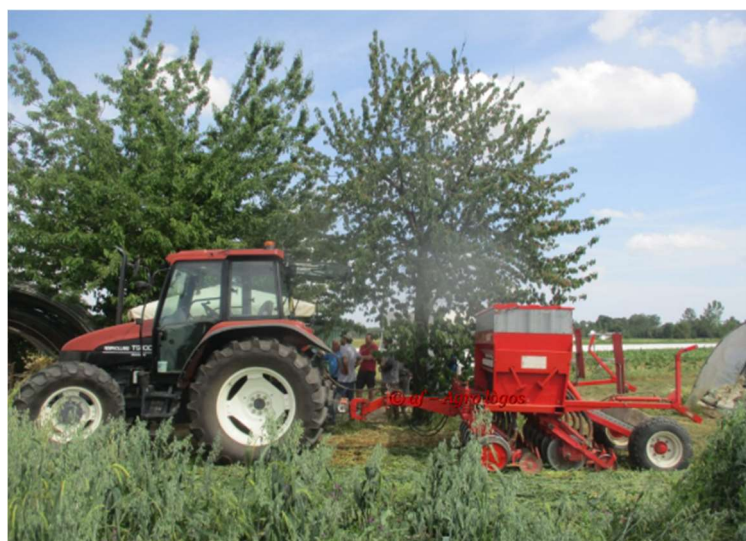
Photo 43, a no-till drill can be used both for seeding a new crop (both cash or cover) and terminate the previous vegetation present at the moment.
