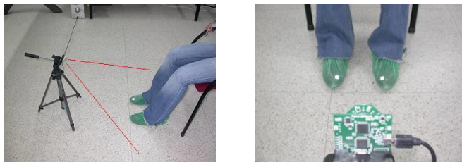
Fig. 1. In the left image, the relative position of the user and the infra-red camera can be observed. The right image shows a view of the reflective markers from the camera perspective.
