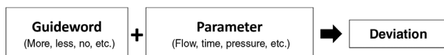
FIGURE 6 Deviation in hazards and operability analysis (HAZOP): the combination of guideword and system parameter
