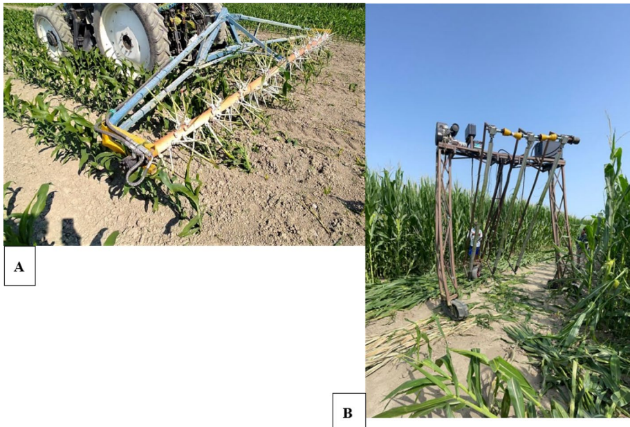
Fig. 2 The two prototypes for simulating hail damages at different crop growth stages used during the two years of experimentation. A Rotating-whip prototype for damaging maize during the early growth stage (8th-leaf stage). B Autonomous vertical rotating pole prototype for damaging maize during the later stages (flowering, milky, and dough) Ph. Lorenzo Carotta
