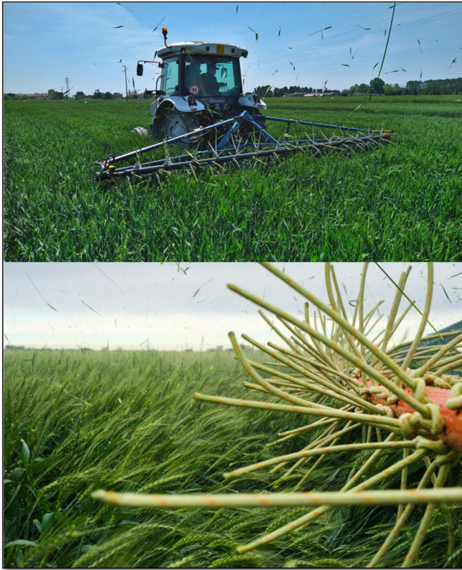
Fig. 2 The designed prototype used for simulating the hail damage at different intensities during the experimentation (above). Below, detail of the rotating ropes system in action during a low damage simulation
