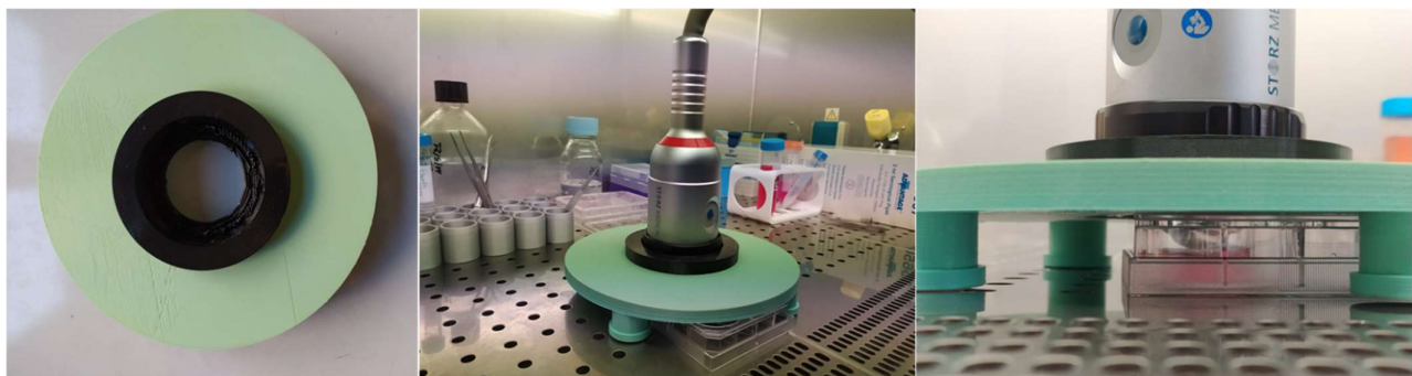
Figure 1. 3D-printed ESW cylindrical coil source support in PVC: the support is composed of two separate top parts (black, which adapts to the coil source size) and bottom parts (green, which keeps the support stable and suspended with respect to the 6-wellplates) were designed using Autodesk Fusion 360 (Autodesk, Inc., San Rafael, CA, USA) to minimize the loss of ESW energy at the interface between head of the device and the 6-multiwells.
