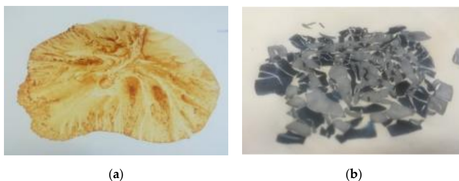
Figure 6. Thin film samples obtained from the 4 mm samples of PEI (a) and PPS (b) after the aging test.
