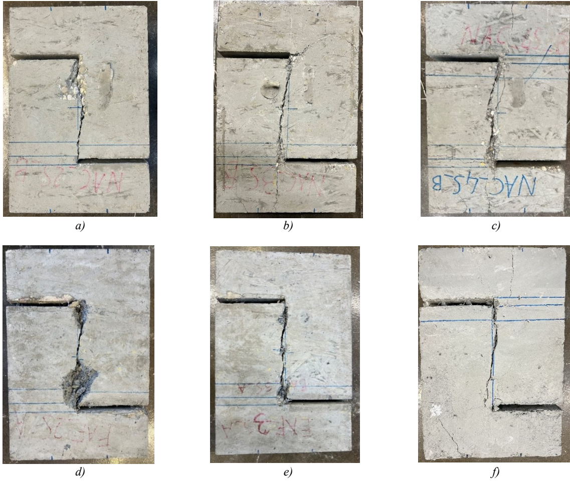
Figure 2-17. Failure patterns in selected push-off specimens: a) NAC-2S; b) NAC-3S; c) NAC-4S; d) EAFC-2S; e) EAFC-3S; f) EAFC-4S.
