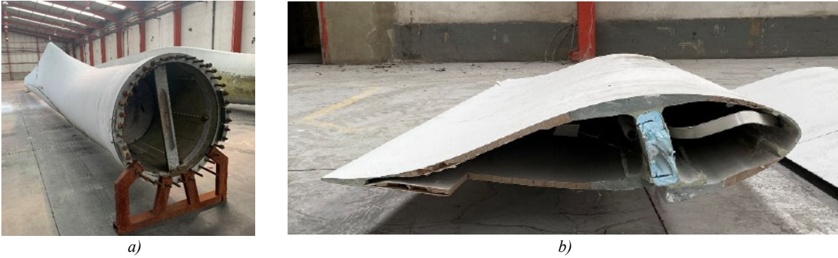
Figure 1-9. Wind turbine blade: a) view of the bolted connection (Source: [112]); b) blade section.
