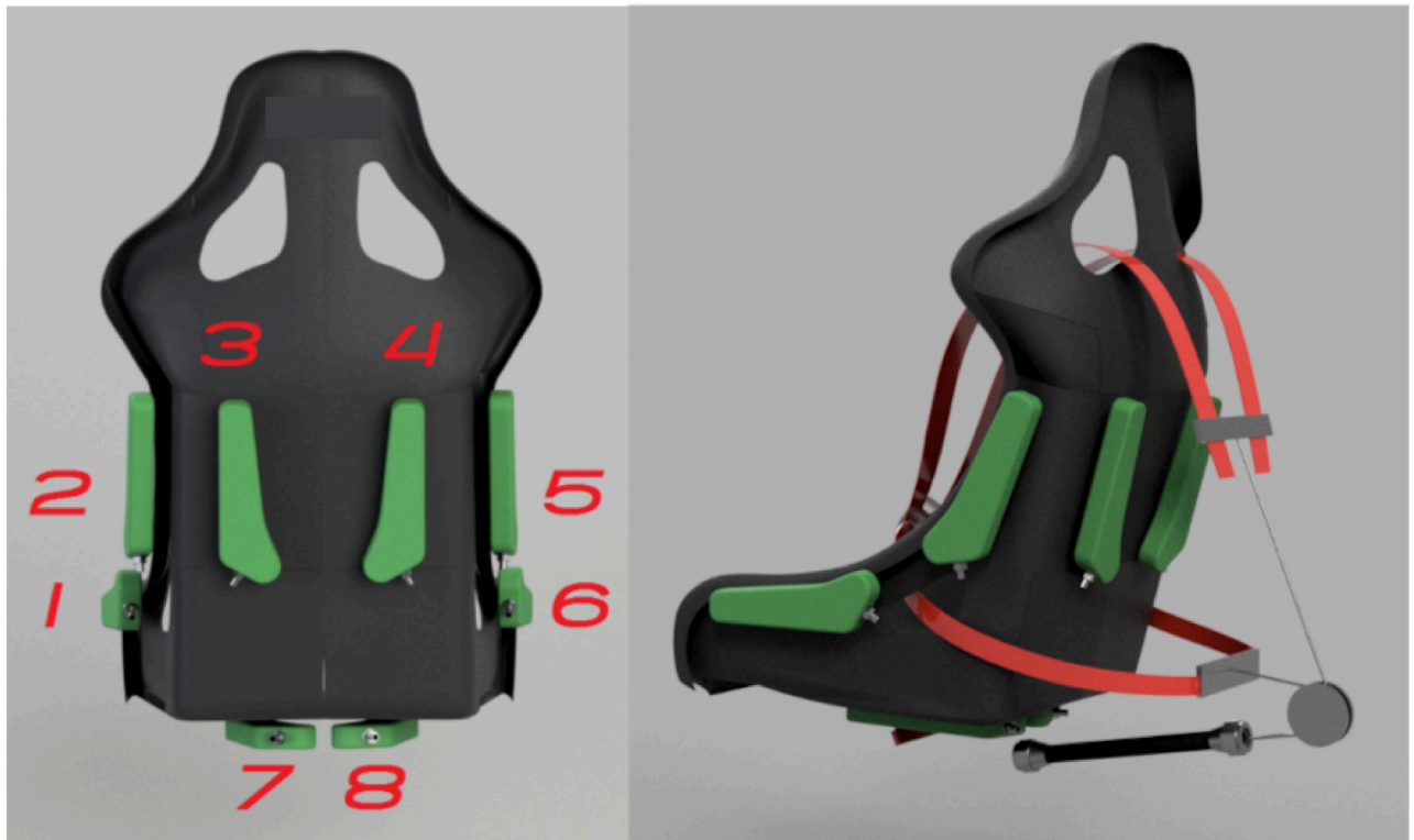
Fig 2. ASB system: The left picture shows the position of the bladders, whereas the picture on the right shows the belts tensioned by a muscle.
