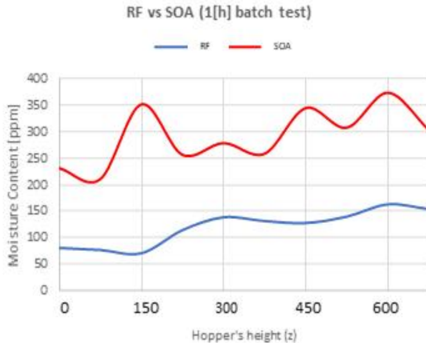
Figure 8.2: Relative Humidity ( RH [%]) along the height of the final prototype. State of Art (SOA) hot air drying vs "new" RF-enhanced drying.
