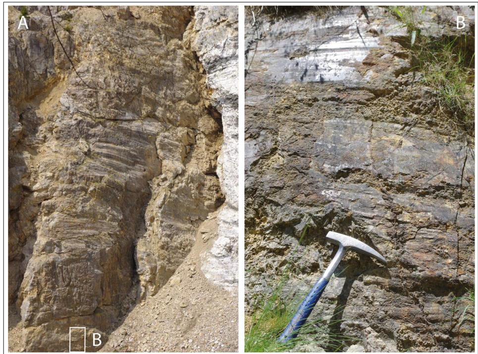
Fig. 7 A Major fault plane in the western wall of the Borcola Quarry with strike-slip lineations (the vertical dimension of the photo is about 20 m). B A close view shows mirror-like surfaces, which are typical of faults in the dolomite rock
