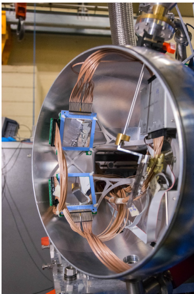
Figure 6. Picture of the experimental set-up for the ^{54}\text{Fe}(^{16}\text{O}, ^{14}\text{C})^{56}\text{Ni} reaction with the two OSCAR telescopes installed in the AGATA scattering chamber.
