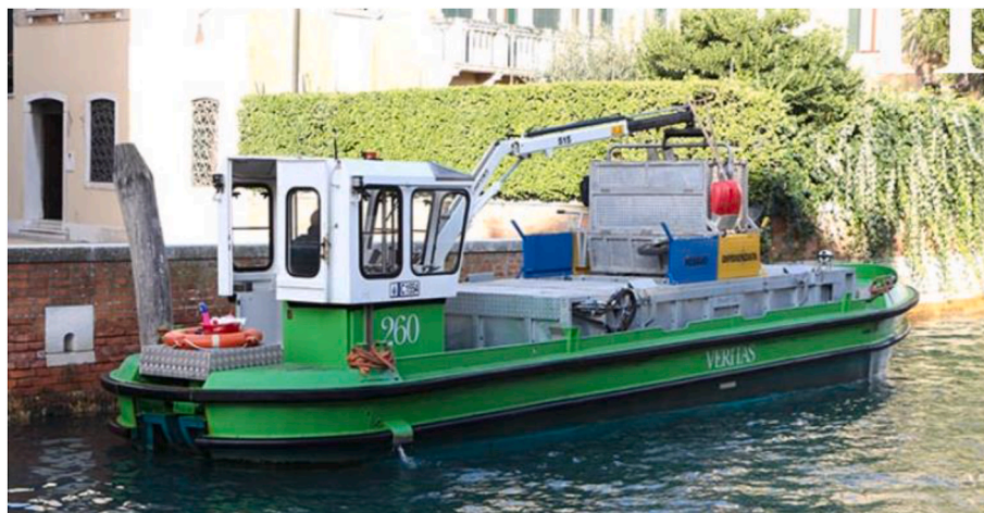
Fig. 2. A Veritas waste-collecting vessel lifting a land bin with the crane and emptying it into the caisson.
