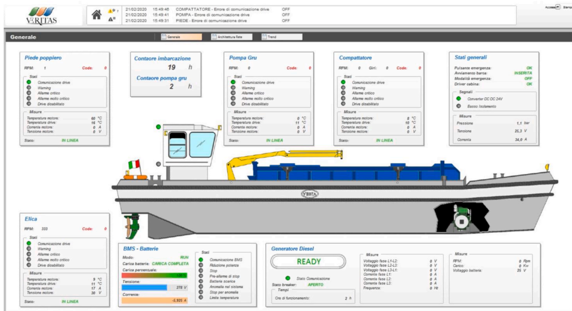
Fig. 10. A screenshot of the remote monitoring system, used for control and maintenance.
