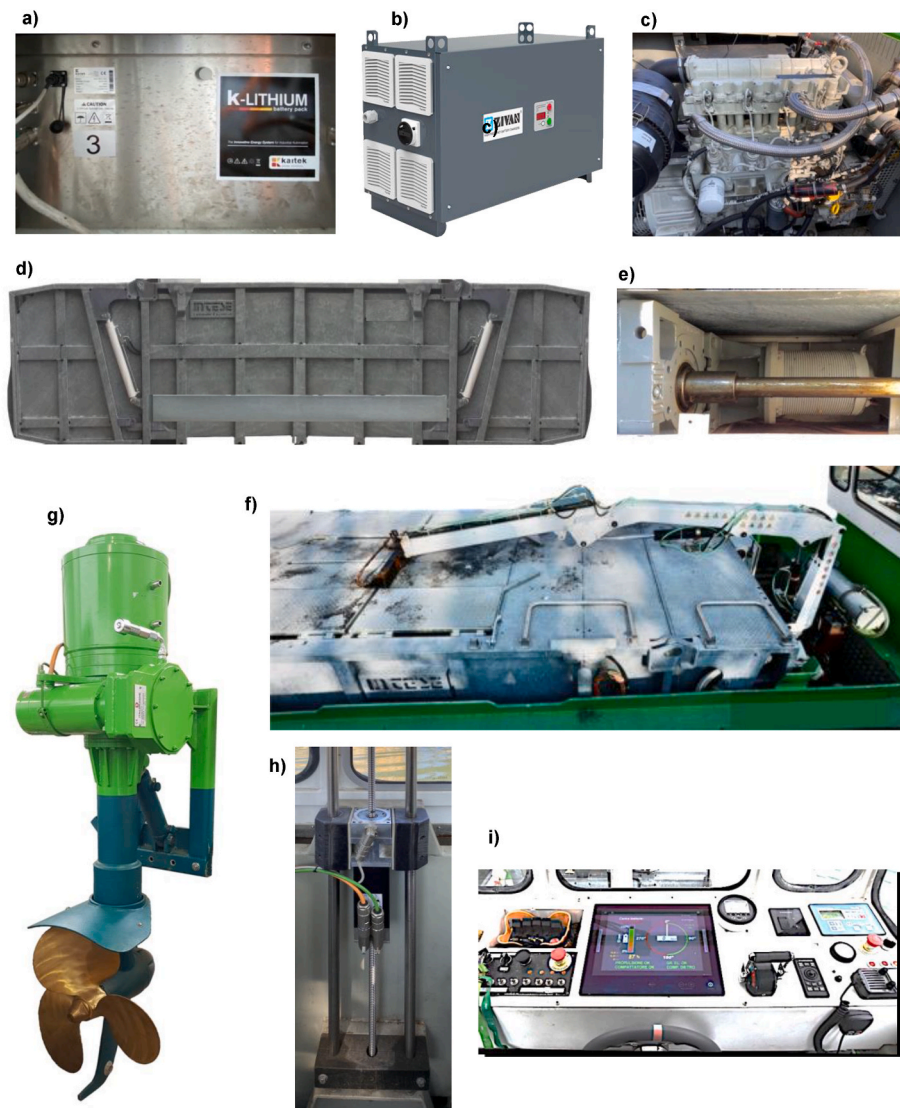
Fig. 8. Components of the PHEB1 (not in scale). a) One of the three modules forming the LiFePO 4 battery by Flash Battery (I); b) 15.4 kW battery charger by Zivan (I); c) Biodiesel generator: 19.4 kW F3M2011 by Deutz (D); d) Waste caisson (lateral view) with e) motor of the two-way compactor (back view); f) Crane laid on the caisson: capable of five movements driven by hydraulic pistons; g) Propulsor: azimuthal IGP-75-01200 by Italdraghe (I); h) Collapsing cockpit: right-hand side drive moving with the cockpit along a worm; i) Dashboard with HMI touch-screen monitor (center), and boat controllers.
