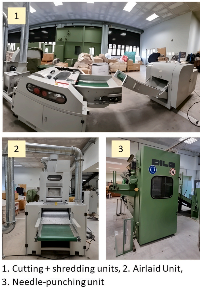
Fig. 1. Detailed configuration of the laboratory-scale mechanical recycling line: (1) Cutting and shredding module for feedstock size reduction; (2) Airlaid unit for web formation and fiber dispersion; (3) Needle-punching section for mechanical web bonding.
