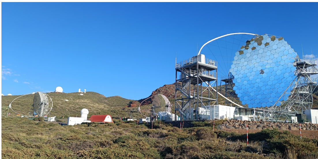
Figure 5.1: Cherenkov telescopes at the Observatorio Roque de Los Muchachos . From left to right, M1, M2 and LST-1.
