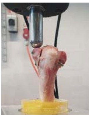
Figure 1: Setup of biomechanical testing, including an ovine tibia cemented in a PMMA potting and load application through a mechanical testing machine.
