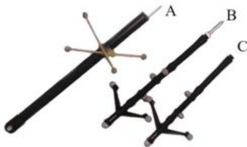
Figure 1: Calibration wands. Wand A is an ad hoc design assembled with hot glue. Wands B and C are 3D printed with a tip machined on a lathe, with C being a slightly shorter design.
