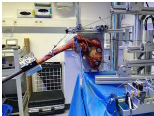
Figure 1: Experimental setup: shoulder specimen positioned at 60° of abduction in the scapular plane.
