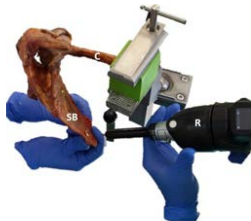
Figure 1: Deflection of the inferior angle into maximum anterior position (SB–scapular body, C–clavicle, R–3D-measuring device)
