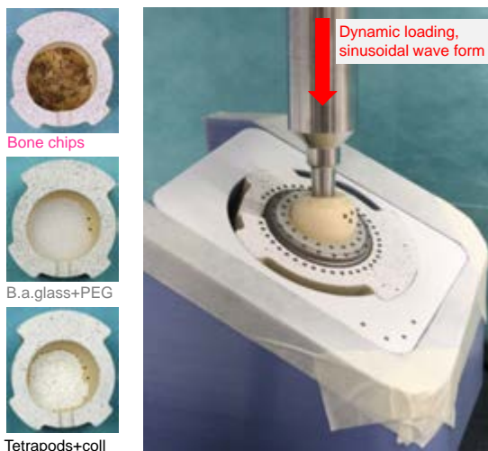
Figure 1: The three test groups bone chips, b.a.glass+PEG and tetrapods+coll in previously developed defect model and exemplary specimen with press-fit cup and tracking points for optical relative motion analysis, dynamically loaded by a servo-hydraulic testing machine.
