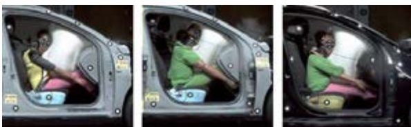
Figure 1: Moment of first contact with frontal airbag (left: Elderly Dummy; middle: HIII 50 th male; right: HIII 5 th female)
