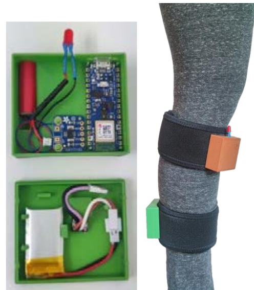
Figure 1: Right, devices position on tibialis anterior peroneus longus and Gastrocnemius muscle. Left, gait event detection system components overview.
