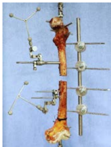
Figure 2: Testing setup to measure interfragmentary motion in cadaver specimens.
