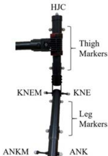
Figure 1: Mechanical leg used for validation. The hinge axis is from KNE to KNEM.
