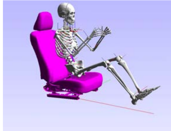
Figure 1: THUMS based MBS model with corresponding coordinate systems at the joints based on PIPER
