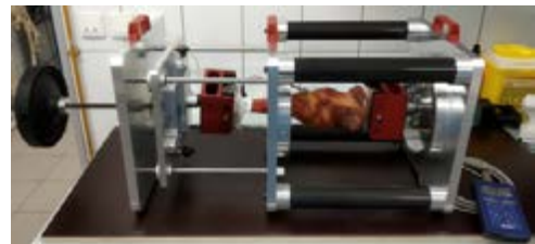
Figure 1. Anatomic specimen and loading setup specifically developed for in situ testing in the CT scan
