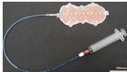
Figure 2: Example of a silicone 3D printed device with a tissue integrating surface topography. [5]
