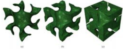
Figure 1: Gyroid models (a) wall thickness 1mm, (b) wall thickness 3mm density, and (c) wall thickness 5mm
