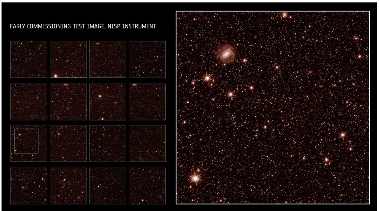
Figure 3.5: First image of NISP in photometry mode taken after the Euclid launch. This was taken using the 'Y' band. This was an image to test if the instrument is on focus and works as expected. The image on the left is the NISP's full field of view, on the right there is the zoom in of the 4% of the full FoV. Credits: Euclid Consortium.
