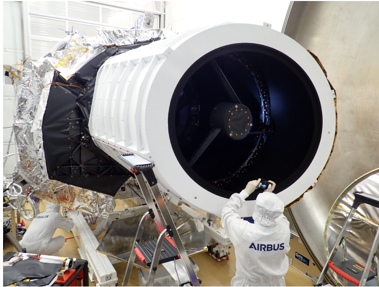
Figure 2.2: The Euclid 's payload, containing the telescope and the scientific instruments. Credits: ESA/Euclid.
