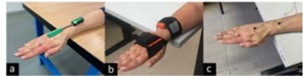
Figure 1: Devices used: (a) Electrogoniometer, (b) IMUs and (c) Micro electromagnetic sensor.
