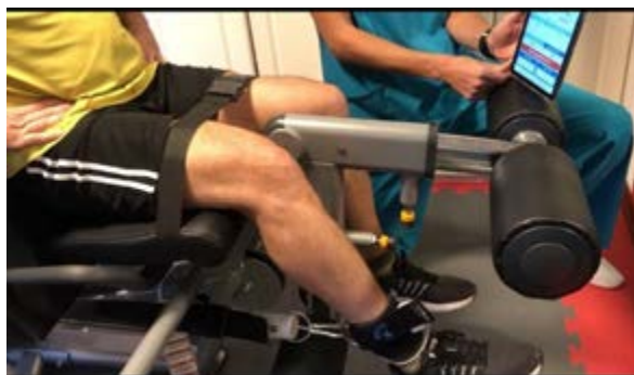
Figure 1: Quadriceps strength measurement as the patient extends the lower limb, with DINABANG secured just above malleolus to a rear fixed point.
