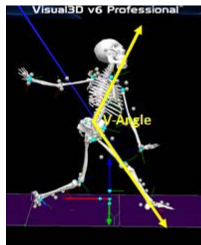
Figure 1: A V-spine flexion angle is calculated between lumbar spine and front shank about the flexion-extension axis of the joint coordinate system.
