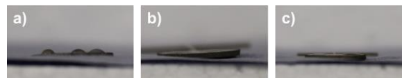
Figure 1 – Water contact angle on Ti-6Al-4V substrates: a) No coating; b) TiO 2 sintered; c) TiO 2 /HAP sintered.
