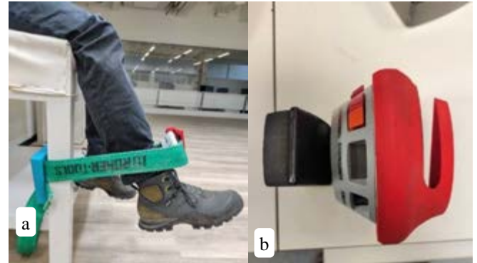
Figure 1. (a) Testing position. (b) 3D printed adapter.
