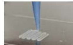
Figure 3: Printing of 2-layer sHAP-PCL composite scaffold. Dimensions of scaffold: 5mm x 5mm x 2mm.
