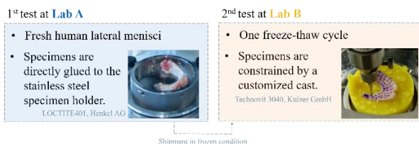
Fig. 1: Summary of the test conditions and fixation methods used in the two Laboratories of this round robin study.
