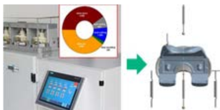
Fig.1: Simplified FE-representation of a wear-testing machine running an HDA-protocol.
