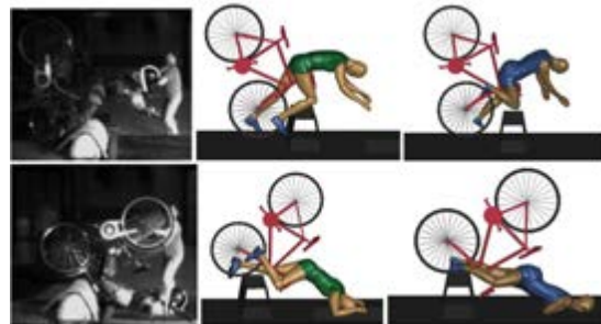
Figure 2: Comparison of kinematics at two instances in time during the barrier collision.
