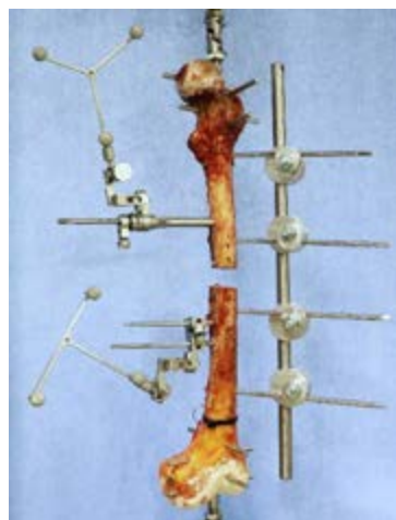
Figure 2: Testing setup to measure interfragmentary motion in cadaver specimens.
