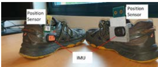
Figure 1: IMU and UWB sensors attached to the shoes of the subject.
