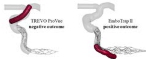
Figure 2: Example of different outcomes with the two tested stent-retrievers for the same patient anatomy.
