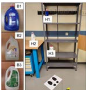
Figure 1: LEFT, bottles used: B1 (2 kg), B2 (3 kg) and B3 (4 kg). RIGHT, scenario with the different heights: H1 (1.5 m), H2 (0.95 m) and H3 (0.51 m).
