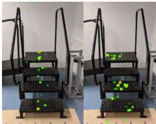
Figure 1: Gaze locations during stair ascent, accumulated from two trials for an able-bodied participant (left) and a participant with transfemoral amputation (right). The colors indicate the duration of each fixation, i.e., the redder the spot, the longer the fixation.
