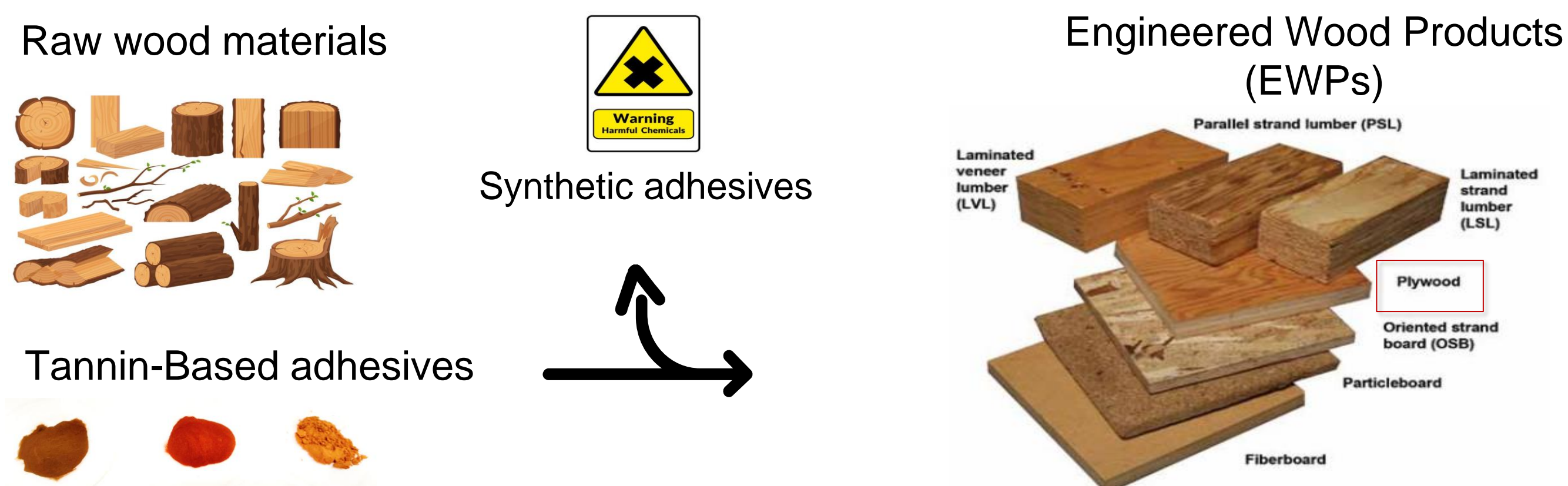
Figure 1. Replace synthetic resins to manufacture engineered wood products through tannin-based adhesive
