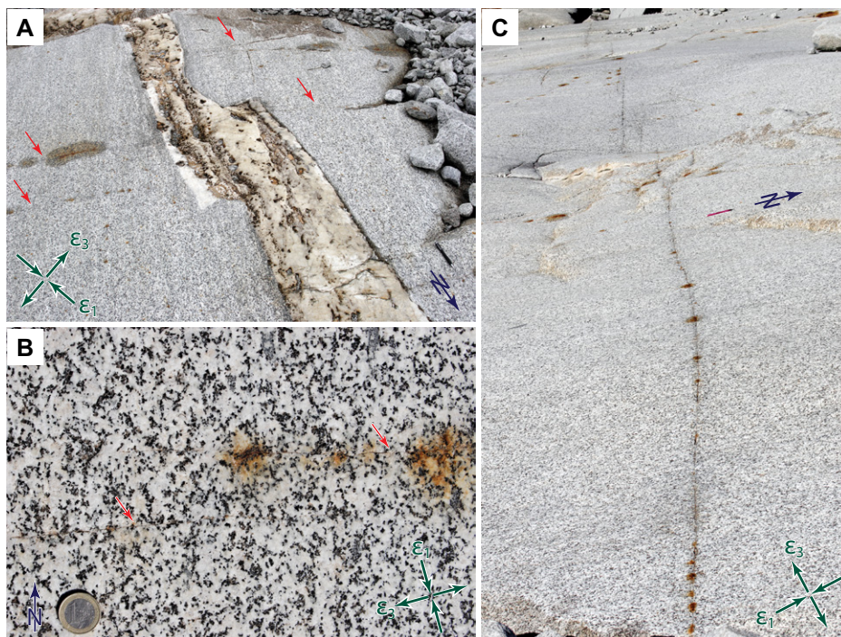
Figure 2. (A) North-south-striking, left-stepping, sinistral quartz-calcite-biotite-plagioclase vein and east-west-striking thin fractures (red arrows). Pen = 14 cm. (B) East-west-striking hairline fractures (red arrows) without discernible offset (joints), showing left-stepping segmentation. 1 Euro coin = 2.3 cm. (C) Overview of segmentation of east-west-striking thin fractures. Pen = 14 cm. Long-term shortening ( \epsilon_1 ) and extension ( \epsilon_3 ) directions are indicated.
