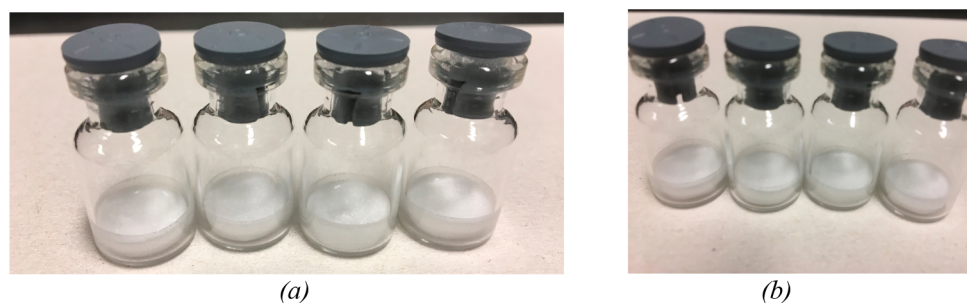
Figure 12. Cake appearance for (a) the central vials and (b) the edge vials at the end of the optimized freeze-drying cycle.
