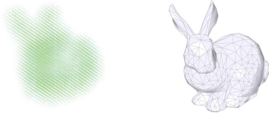
Figure 11. SDF of a geometry structures and its .STL format geometry.
